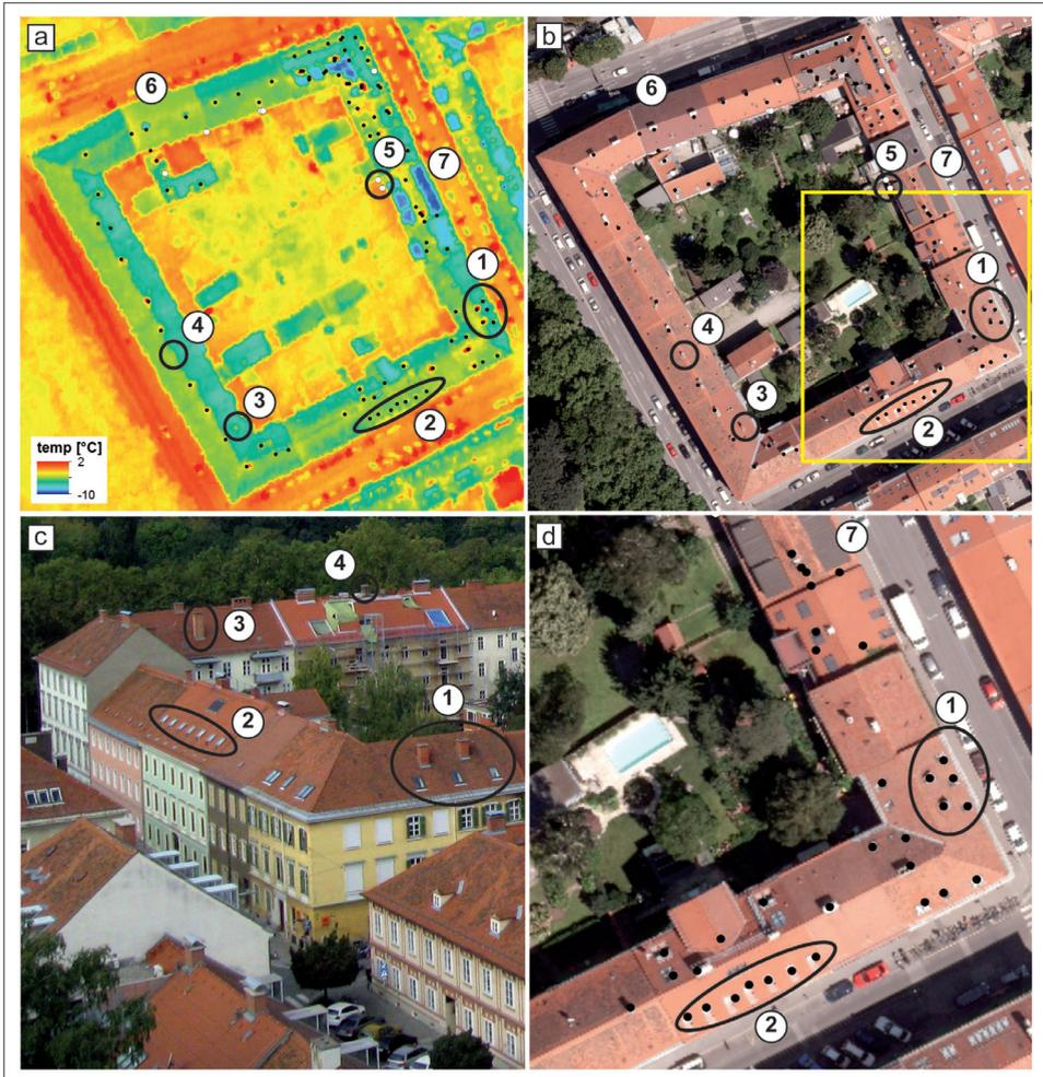
Position 1 and 2 indicate a precise relationship between expected and detected hot spots (chimneys and roof windows). Position 3 and 4: Chimney which does not achieve the required algorithm criteria. Position 5: Example of an excluded hot spot within the minus 1m buffer distance of the building envelope.
